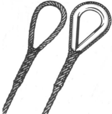
② Mechanical Splice/Talurit
